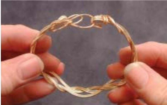
Place either flat-nose or chain-nose pliers about halfway between the wrap and the cut ends and bend the four wires into a hook-shaped clasp (**Figure 54**). *Work slowly.* If you bend the wires down from just one side, the clasp will be crooked. Bend the wires down from the left side a little (**Figure 55**), then reposition the pliers on the right side and bend down a little more (**Figure 56**). Work back and forth until the wires form an even clasp (**Figure 57**).
